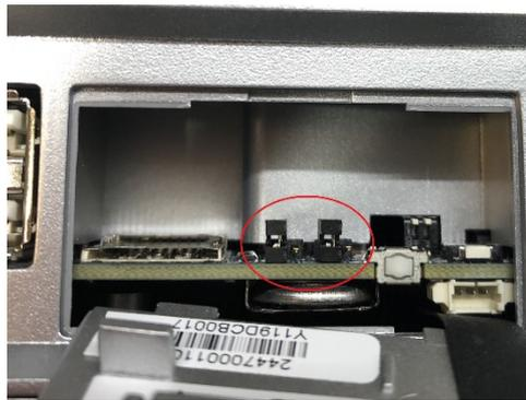
Open service panel with jumpers in correct and wrong orientation
