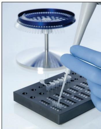
2. Place the Caps securely on the Strip Tubes and visually inspect to confirm a tight seal.
