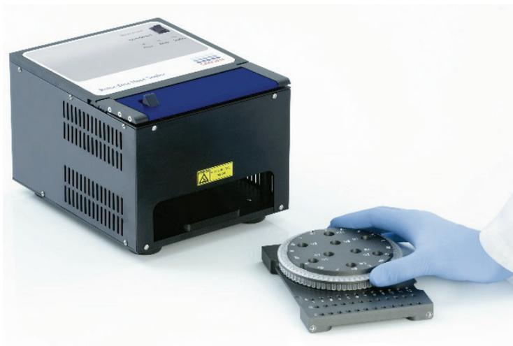
5. Take one sheet of Rotor-Disc Heat Sealing Film and remove the smaller circular cutout in its center by slightly folding the film in half without creasing, pinching the central piece and carefully tearing it out.
