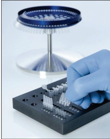
3. Insert the Strip Tubes into the 72-Well Rotor, ensuring that each tube sits correctly in place in the correct orientation. Samples will not be optimally aligned over the detection system if not placed correctly in the rotor. This could result in a reduction in acquired fluorescence signal and detection sensitivity. A Rotor Holder that enables easy tube loading is provided with the instrument.
