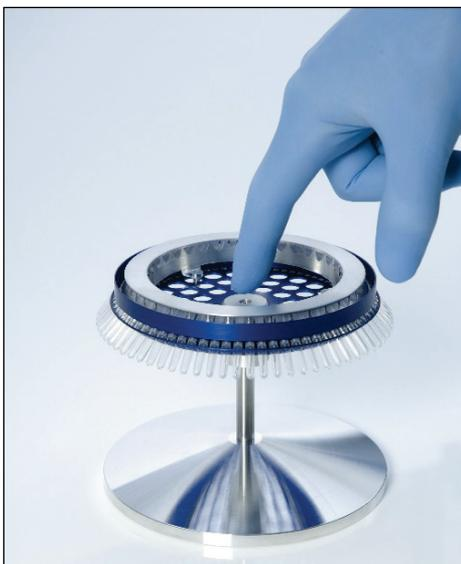
5. Insert the assembly into the Rotor-Gene Q MDx chamber by clicking into place using the locating pin on the rotor hub. To remove, simply push down on the rotor hub to release and pull out.
