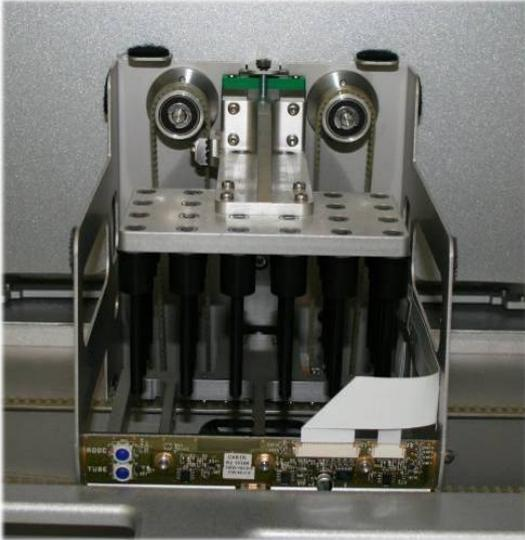
3. Wipe the exterior of the magnetic head with a lint-free cloth moistened with ethanol-based disinfectant (e.g., Mikrozid), and incubate as appropriate.
