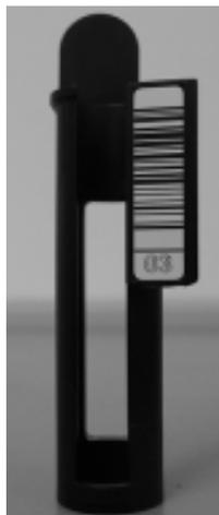
**Example of insert for tube carrier.**
