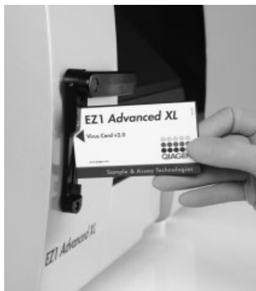
Figure 4. Ease of protocol setup using EZ1 Advanced XL Cards. Inserting an EZ1 Card, which contains a protocol, into the EZ1 Advanced XL instrument.
