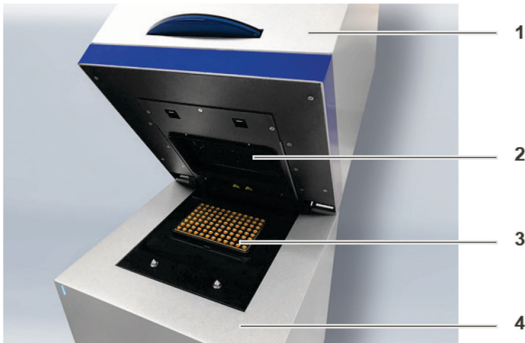
Figure 1. Layout of the QIAquant 96. 1: Upper part with fluorescence photometer and integrated tablet, 2: heated lid, 3: sample block, and 4: thermal cycler.
