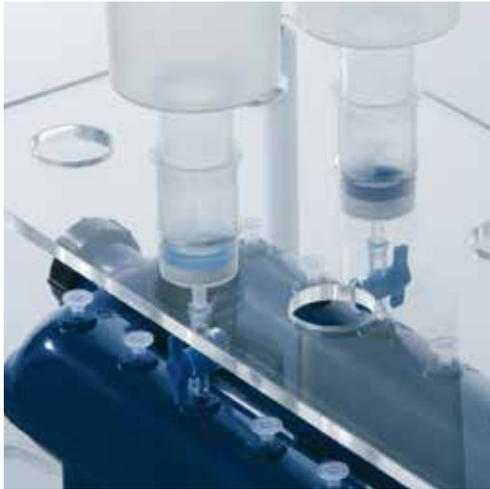
**Figure 1. QIAGEN Plasmid Plus Mega and Giga columns on the QIAvac 24 Plus.**
